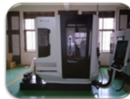
DMG MORI make, CMX 600V Vertical Machining Centre With 3D-control HEIDENHAIN TNC 620 with ASCII keyboard (15" TFT) Control System.
